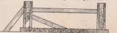
Below—Method of bracing shuttering for walls
