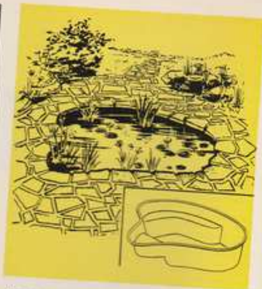
Above: Easy to install are the fibre-glass ponds such as illustrated here. Paving or rocks are used to conceal the edges of the tuckered pond.
