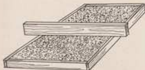
Above—Use a long plank to tamp base (posts on shuttering not shown)
