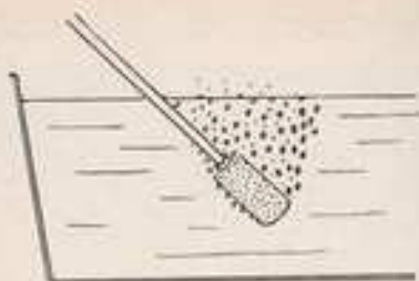
By using a diffuser stone and aerator food particles can be kept moving
