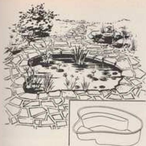
Easy to install are the fibre-glass ponds such as the Leedale (Charplex Engineering Co.) illustrated here. Paving or rocks are used to conceal the edges of the sunken pond.
