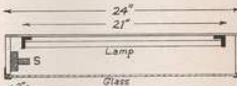
Section through light hood to show arrangement and sizes of tube and starter (S); ballast choke is not shown.
