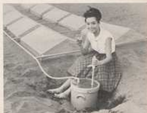
What is in effect distilled water collects in the pipes from these "greenhouses" when the sun's heat causes evaporation from the soil.
