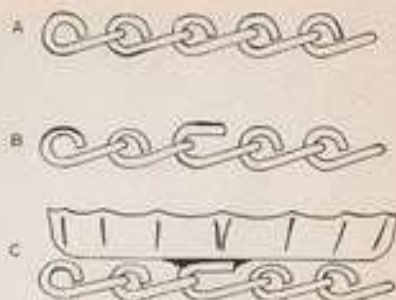
Fig. 3. In B an end link of the chain A is shown opened for attachment to the end of another length of chain. C, side view of bottle cap soldered to a link of the chain for use as food container
