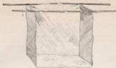
Muslin bag on wire frame, used by the author to contain Daphnia used for clearing green water and for feeding with small specimens.
