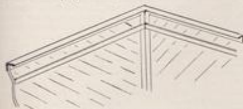
View of inside of top of one aquarium corner showing glass strips in position
