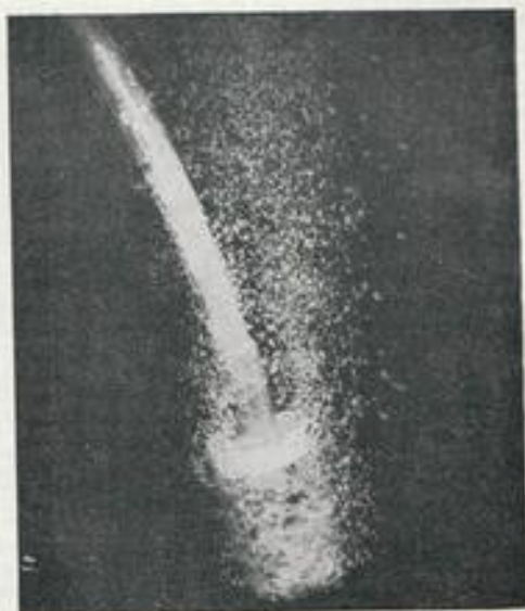
Porous stone "diffuser" at end of aerator line
