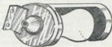
Screw-lid tin adapted as a lamp-holder
