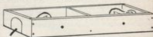
Wooden base of the aquarium housing the lamps, which are mounted on the end "doors." A view of the finished aquarium is shown at the top of the page
