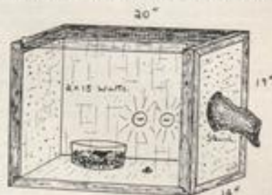
An easily constructed fly breeding case lighted and heated by two low-wattage lamps.
