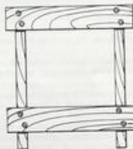
End view: This shows the table like construction make the top the exact width of your tank.
