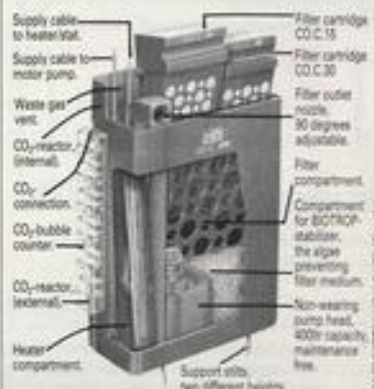
A two-cartridge filter makes the management of nitrification and de-nitrification relatively easy to handle.
