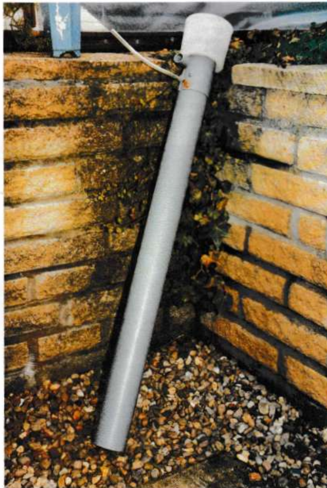
Foam fractionation in the UK is not taken seriously, but we must be the only ones with our heads buried in the sand. The photograph shows a venturi driven fractionator.
