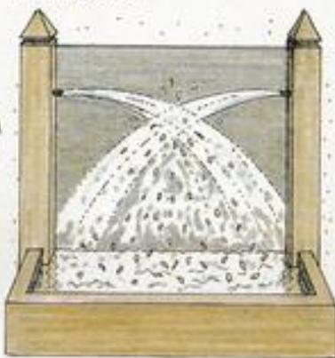
Opposing fountain jets form a splashing spectacle, fixed in timber posts with a slate slab back, the water drops into a shallow timber basin lined with butyl rubber to be recycled through the jets.
