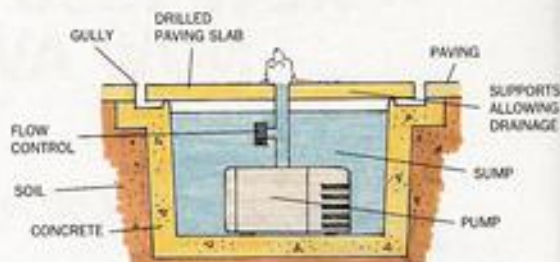
Diagram showing a cross section of a flat fountain using a drilled paving slab placed over the sump holding the pump.
