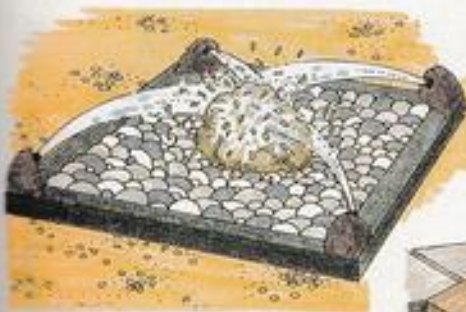
▲ This square feature has a fountain jet placed at each corner to splash onto a central stone, the water drains into the pebble base to be pumped through the system again. The whole is set in gravel.
