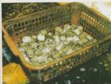
Sintered glass medium in a dealer's vat. This is used by many dealers as a means of effectively eliminating nitrite, which can be very persistent in environments where the stocking level is continually changing.
