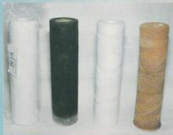
This picture shows graphically the value of prefiltration in a purifier. The cartridge on the extreme left is an unused one, the one second left is from the purifier prefilter of a keeper whose water suffers from high sedimentation. Third left is a new dechlorinator prefilter cartridge, and, lastly, the same cartridge type from a low sedimentation area after over 500,000 gallons of water has gone through it.
