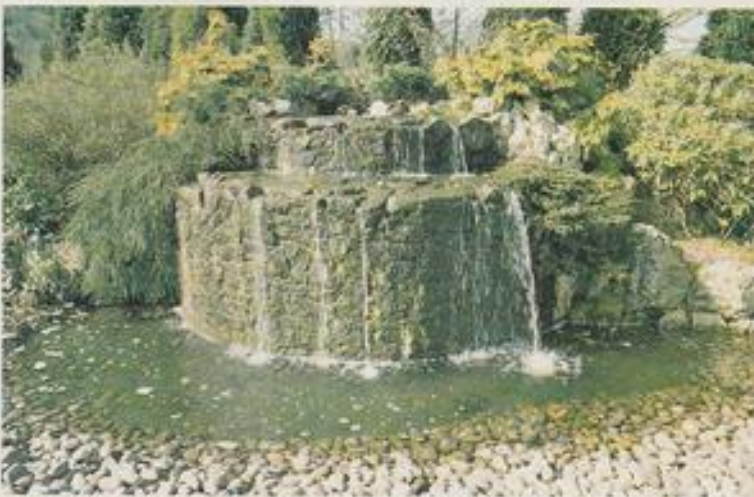
For this type of waterfall effect, allow 50-60 gallons per hour to the height you want for every 1 inch of width of spill.
