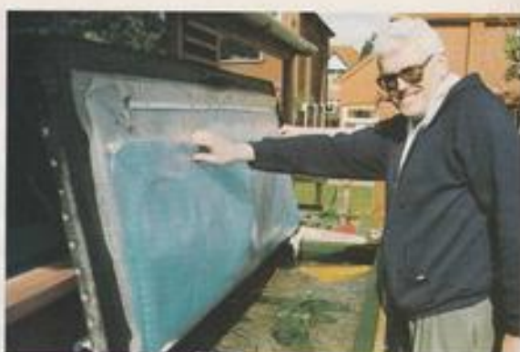
This is the outside filter. Because of its situation, outside the shed, you will note that it is very heavily insulated. The brush chamber is nearest to us, and the biological chamber beyond. Note the airlines which feed airstones situated within the filter.
