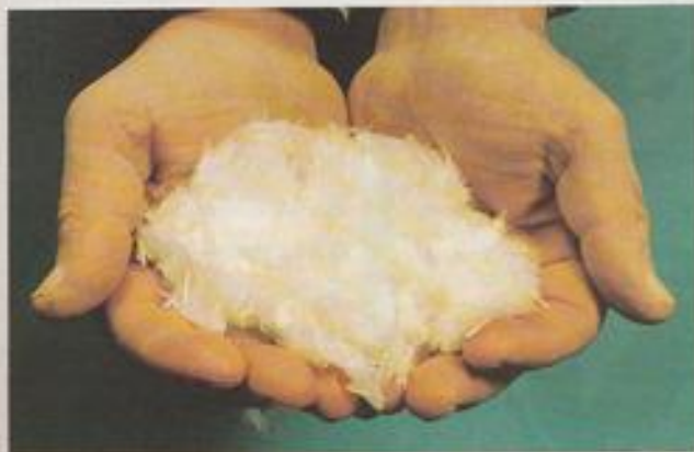
This is Fibromix. These glass fibres are mixed evenly in the rendering to help prevent cracks forming.
