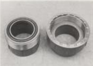
Union dismantled to show the rubber seal.
