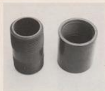
Reference is often made to male and female threads. This picture shows the difference: (left) male thread; (right) female thread.
