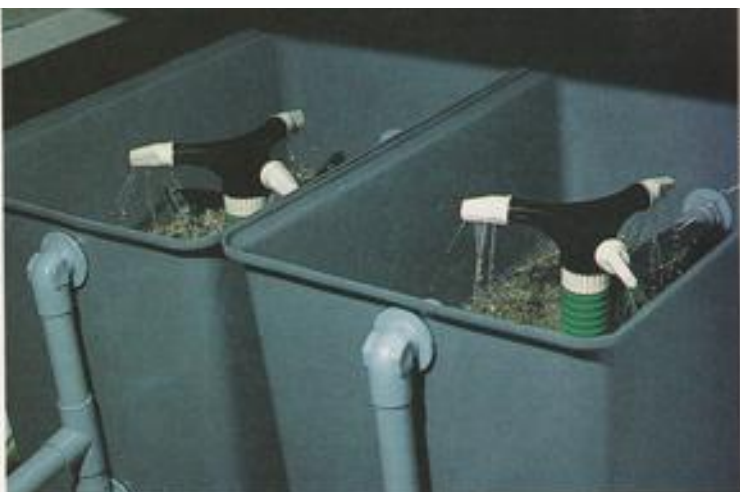
Filter design offers great scope for creativity. In this case these out-of-pond filters have their water supplied via rotating lawn sprinklers.
