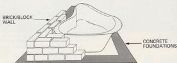
Prefabricated ponds can be installed fully sunken, or, as in this case, raised, with a surrounding brick/block wall built on solid concrete foundations. Diagram reproduced from John Dawes' Book of Water Gardens (TFH Publications, ISBN: 0-86622-662-1).
