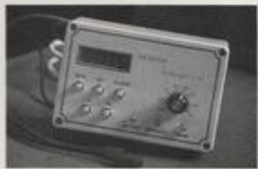
Modern external thermostats can be located away from the aquarium or vivarium and can even incorporate an alarm.
