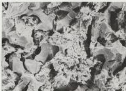
SIPORAX ® surface structure, enlarged 300 times, inhabited by sessile bacteria. Correct use ensures control of ammonia, nitrite and nitrate.
