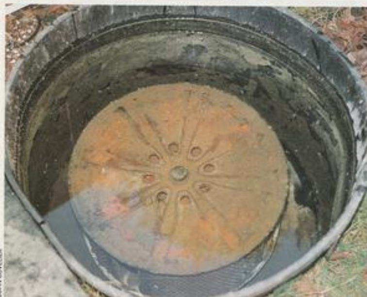
My home-made pre-filter consists of a stainless steel washing machine drum filled with hair rollers. The feed pipe comes into the base.
