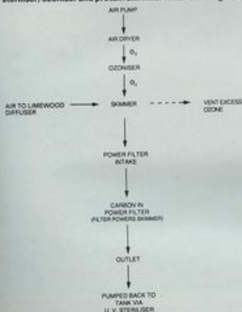
Flow chart showing the sequential installation of UV steriliser, ozoniser and protein skimmer when used together.
