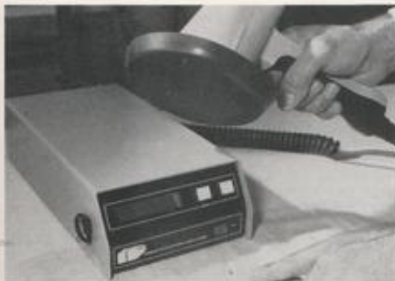
Above left, identification of the micro-chip code is carried out with a transceiver and scanning device. Above right, the chip is sterilised before being inserted by means of a hypodermic in a two-minute operation.
