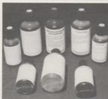
Above: Copper Test Kit distributed by Technical Aquatic Products includes simple pictogram instructions and clear colour comparator scale
